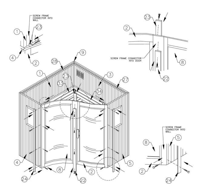
Figure 5. Attaching the front wall with door
